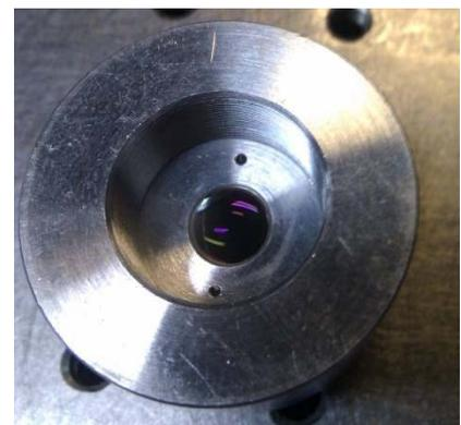
Figure 7 - Focusing optic plate
