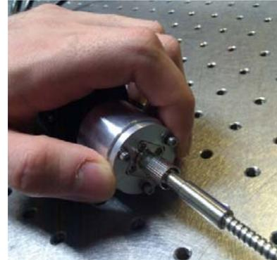
**Figure 5 – Adjusting the coupler plate**
