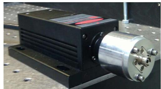
Figure 2 - A Laserglow Technologies 473nm LabSpec laser module with optical fiber coupler attached
