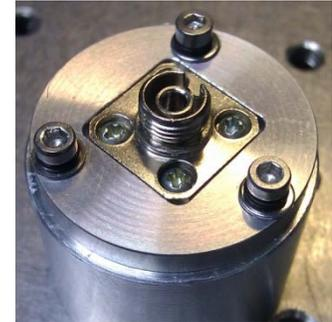
Figure 1 - An optical fiber coupler
