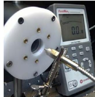
**Figure 4 - Measuring laser output power with and without fiber**
