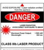
This device is compliant with 21 CFR1040.10 and 1040.11 LASERGLOW/COM LIMITED, 873 St. Clair Ave. W. Toronto, ON, Canada M60.104 Manufactured: 07-2012, Toronto, Canada
